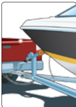
A bow safety chain holds your boat if the winch fails.
